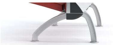
The front and rear leg are incorporated in a single arch shaped casting. The arch is formed in a T-Shaped profile to achieve stiffness and strength with minimal weight and a slim appearance. The legs bolt to the T-Slot grooves on the bottom of the beam. Each leg casting includes 2 die cast adjustable glides. Optional anti-slide glides or floor-fastening glides are available for hard surfaces.
