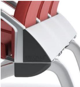
The supporting beam is made from a robust 5 1/4" x 4 3/8" (130mm x 110mm) triangular aluminum extrusion with 3/16" (4.8mm) thick walls. The beams are heat treated to T5 temper for maximum strength.
